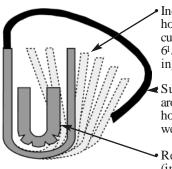
• Indestructible, flexible aluminum hooks adjust wider or narrower to custom-fit and grip items up to 61/2" deep. Soft Neoprene covering won't mar equipment.
